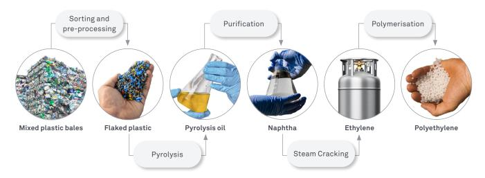
Figure 1. Process flow to chemically recycle mixed plastic waste to virgin quality polyethylene.
